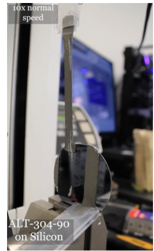
Figure 10: 180 Degree Peel Adhesion Test Set up and Results
