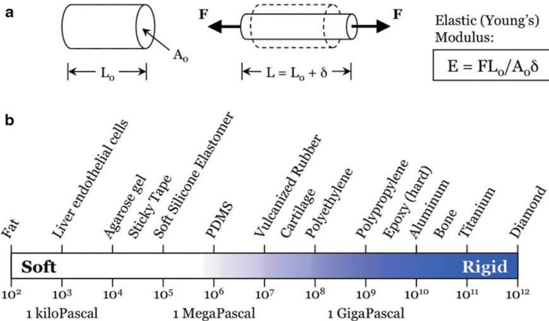
**Figure 1:** (a) The elastic (Young's) modulus scales with the ratio of the force  $F$  to the extension  $d$  of a prismatic bar with length  $L_0$  and cross-sectional area  $A_0$ . (b) Young's modulus for various materials.<sup>ii</sup>
