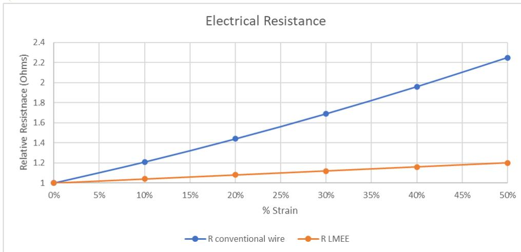
Figure 2: Resistance when strained
