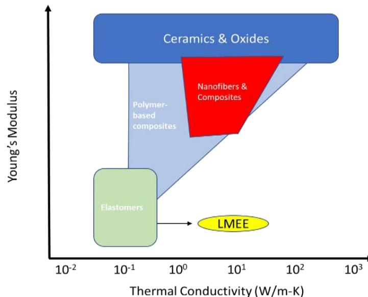
Figure 3: Thermal Conductivity – Conformability Trade-off
