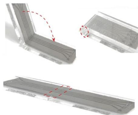
**Figure 4:** LMEE connections in a hinge application
