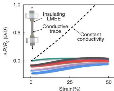
**Figure 3:** Normalized resistance as a function of strain
