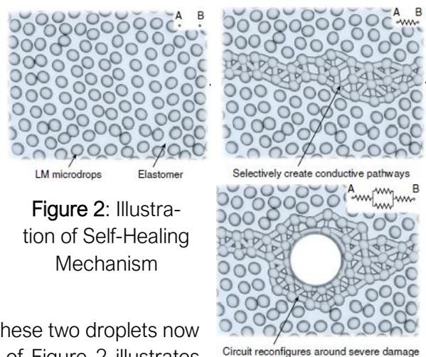
**Figure 2:** Illustration of Self-Healing Mechanism
