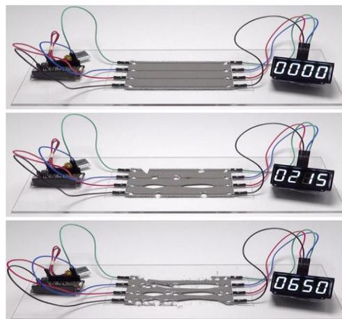
**Figure 5:** Recreation of electrical circuits around severe damage
