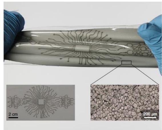
**Figure 1:** LMEE Composite with conductive traces
